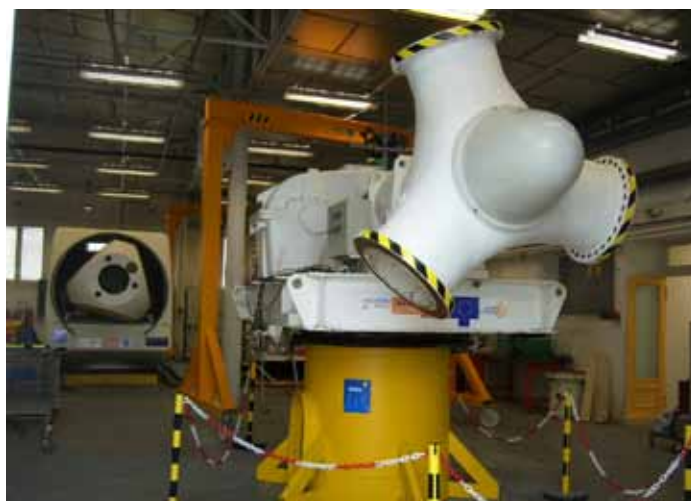
Figure 1 - 250kW training turbine on a pedestal mount at a BZEE partner college
